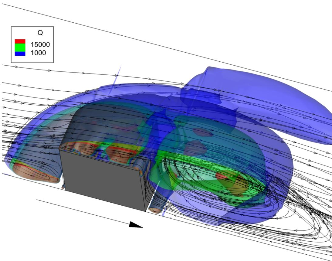
1 Q-criterion isosurfaces represent local balance between shear strain rate and vorticity magnitude.
