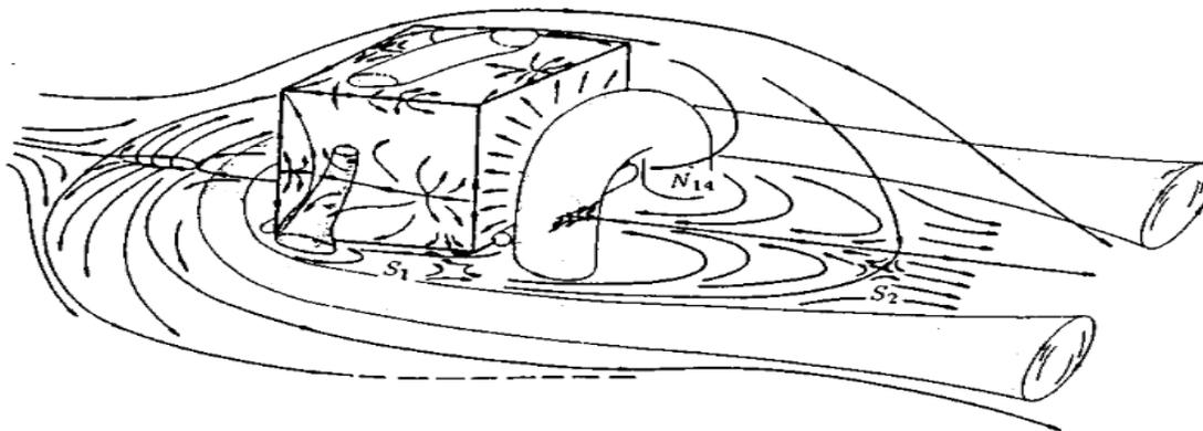
The vortex system starts at the leading edge of the cube with a horseshoe vortex extending along both sides of the obstacle, a large arch vortex at the trailing edge, and a separated flow with associated vortices along the top face of the cube. The following figure shows the flow structure computed by Coolit showing Q-criterion<sup>1</sup> isosurfaces outlining the vortex structure with the section along the channel centerline.
